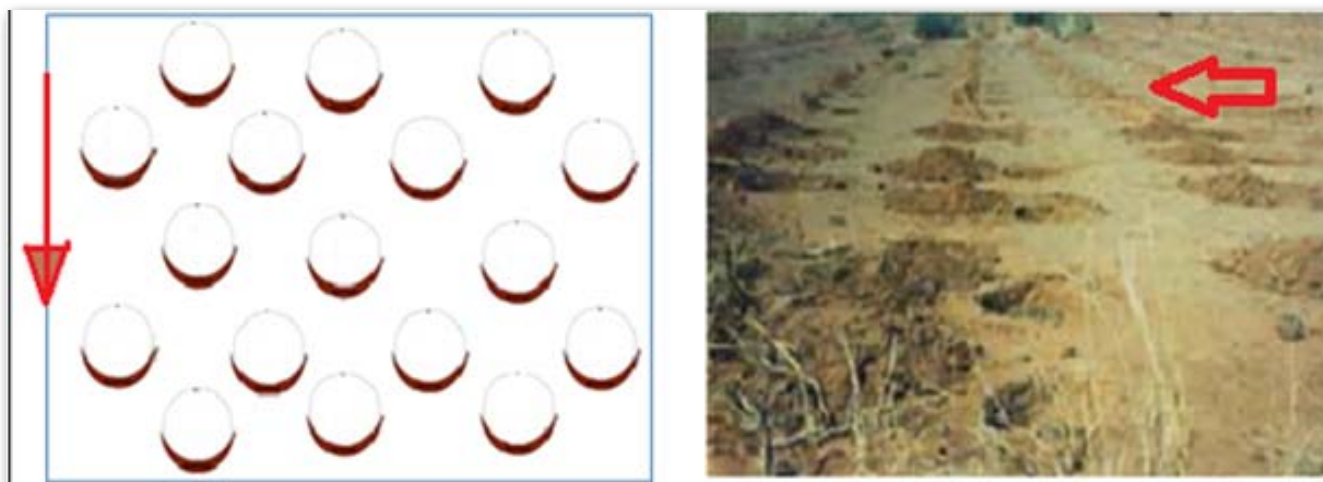
Fig 6.4 Staggered design and construction of zai pits in moisture stress area
