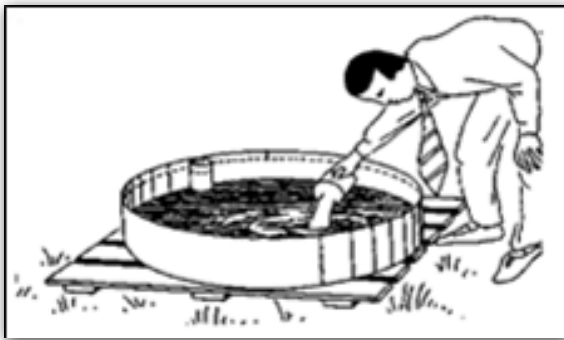
Fig 19.8: Adding water when water depth in the pan drops too much
